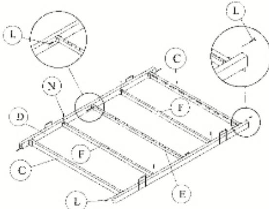
**Step 1** Fix both side rails D and cross bar E with bolt L as above diagram. Put cross bar F into side rail and fix in bolt N. After that put end cross bar C to the end of side rail and tighten with bolt L.
