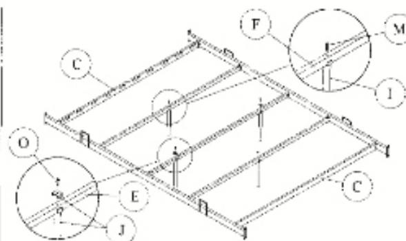
**Step 2** Fix bed support legs as shown on the picture.
