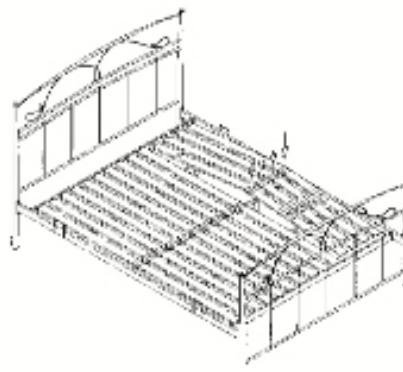
**Step 4** Once wood slats have been inserted into the plastic caps, fix one end of wood slat into the hole of end cross bar C and the other end to the other end cross bar. After that fix the plastic cap to the center cross bar by pressing it accordingly to the default holes. Ensure the plastic cap's pin aimed to the hole.
